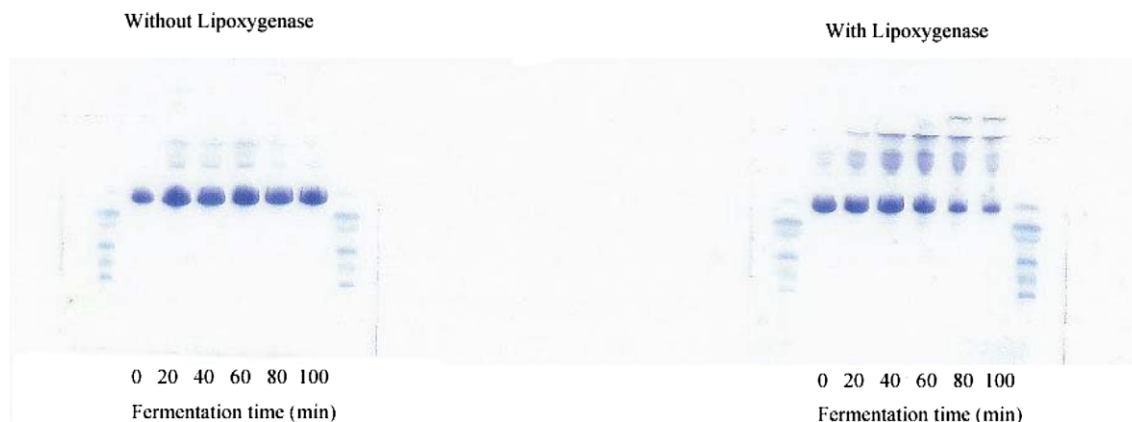
Fig. 7. Changes in the molecular weight of gluten when dough was fermented for 100 min.
